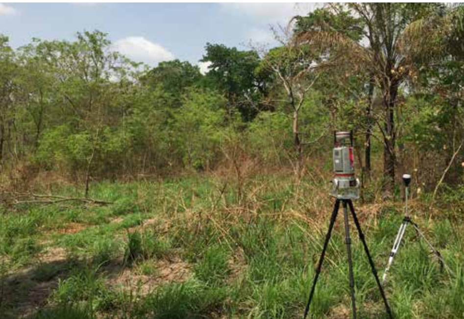
Measurement of the structure of tropical forests and their carbon stock using terrestrial lasers - location: Ghana (image: Christian Budach/GFZ).
